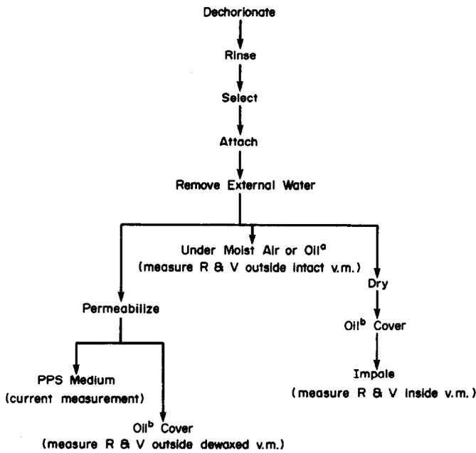
FIG. 1. Protocols for preparing eggs for various measurements. (a) Mediflor; (b) halofluorocarbon oil; v.m.: vitelline membrane; PPS: polar pocket simulant.
