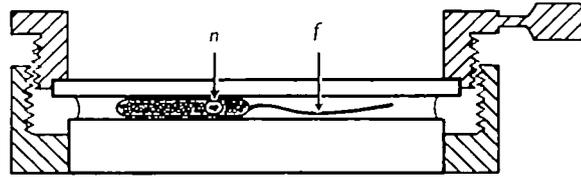
Fig. 1. Diagrammatic cut-away view from the side of the rotocompressor containing a *Peranema* flattened to about the diameter of the nucleus. The cell is in a drop between two circular pieces of glass (not cross-hatched) mounted in separate metal holders (cross-hatched) which screw together. The size of the *Peranema* (and the metal threads) relative to the size of the rotocompressor is greatly exaggerated in this diagram and in Fig. 2. (*f*, flagellum; *n*, nucleus.)
