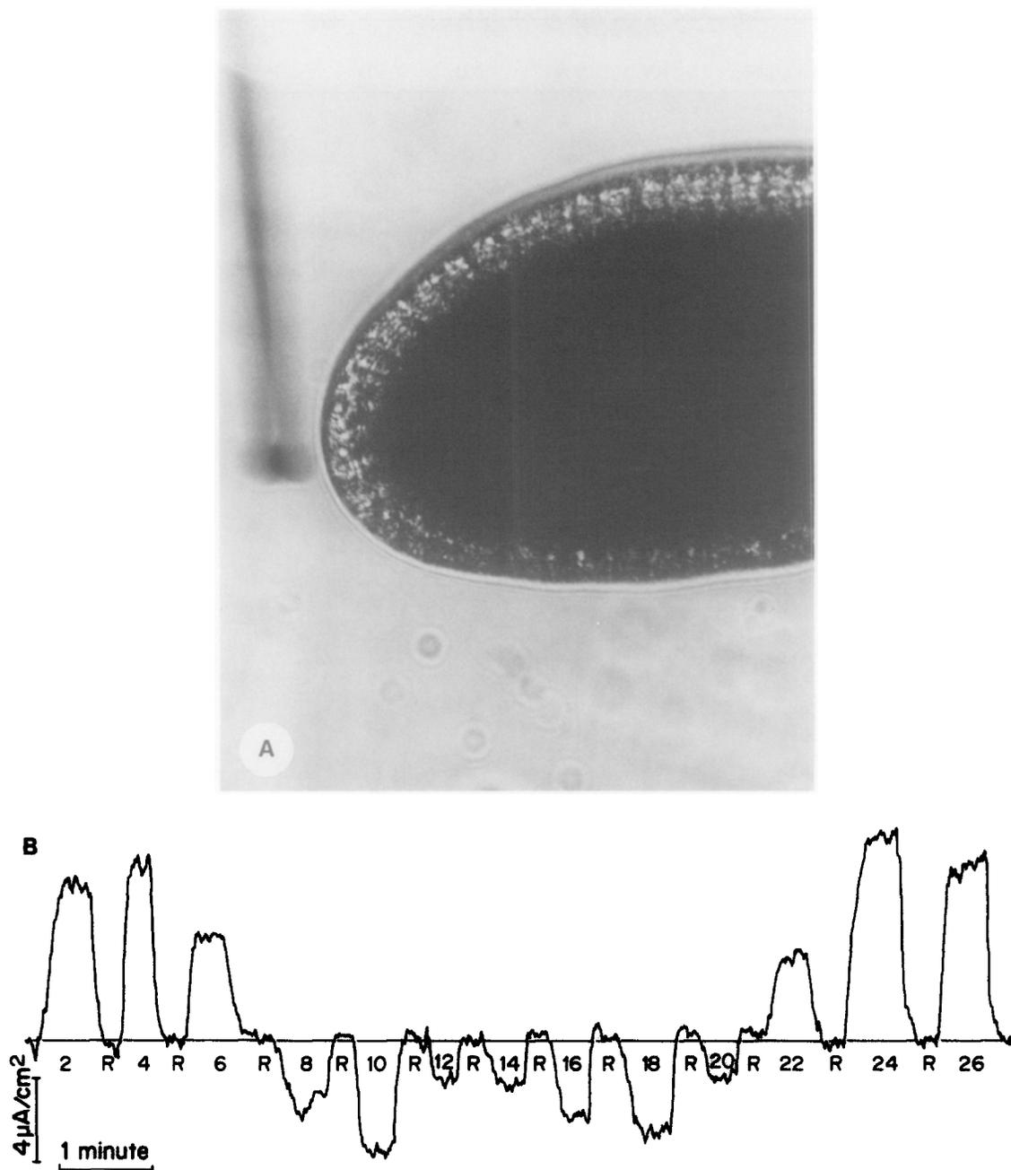
FIG. 2. (A) Vibrating probe in a position to measure current normal to the rear pole of a stage 10 follicle. (B) Record of current densities entering or leaving stage 11 follicle 14. An upward deflection represents inward current. After each measurement, the probe is returned to a reference position (R)  $300 \mu\text{m}$  from the follicle to establish a zero current baseline. Every second measuring position is presented here. A map of the full record is shown in Fig. 4.
