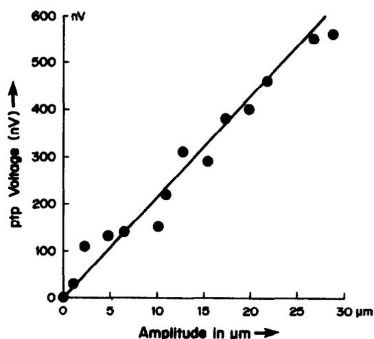
FIG. 3. Peak to peak voltage versus vibration amplitude. Measured with the probe as close as possible to a stage 10A follicle in a lateral position. Its distance from the follicle was smaller than those used in routine current mapping. The data indicate an outward current of  $4.2 \mu\text{A}/\text{cm}^2$  independent of vibration amplitude.
